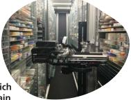
As well as dispensing medicines at twice the speed of the previous robot, and being able to pick multiple packs at once, the new robot also reads 2D bar codes which allows it to issue the packs in the correct expiry date order. Previously staff had to manually check the expiry dates and put them back into the machine in the correct date order.
