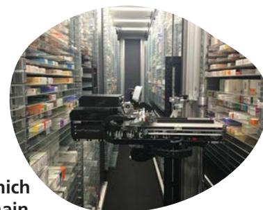
As well as dispensing medicines at twice the speed of the previous robot, and being able to pick multiple packs at once, the new robot also reads 2D bar codes which allows it to issue the packs in the correct expiry date order. Previously staff had to manually check the expiry dates and put them back into the machine in the correct date order.
