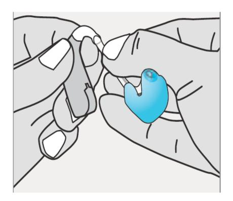
4. The curve of the earmould should line up with the curve of the hearing aid.
